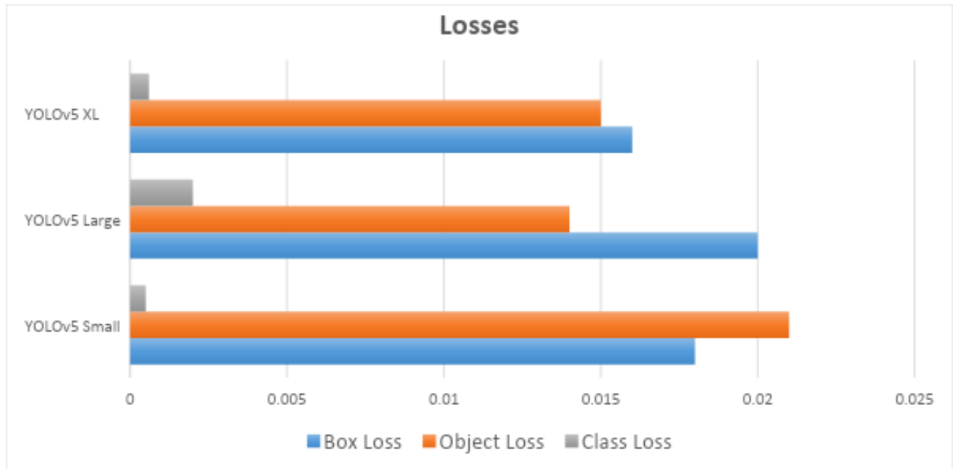
Fig. 29: Loss score Comparison of different YOLOv5 architecture
