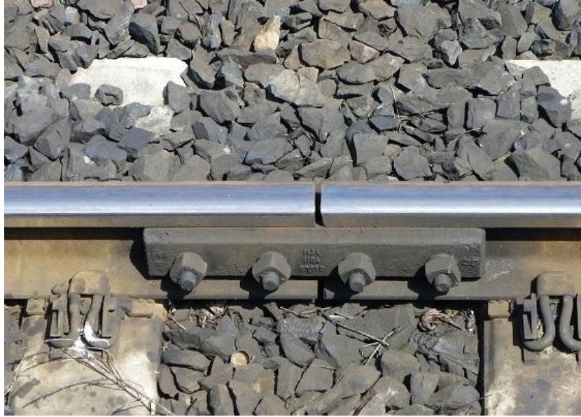
Fig. 3: Structure and Operating Location of Fishplates
