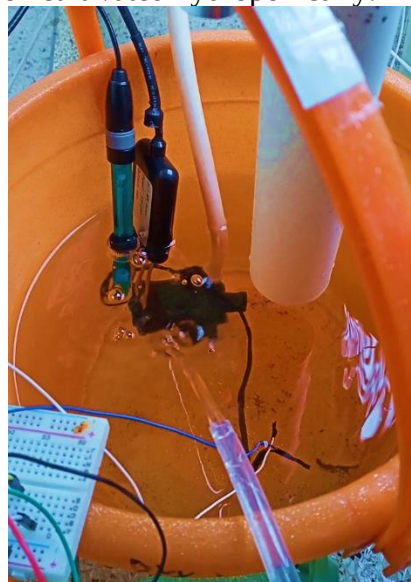
Figure 2.18: pH Control & Monitoring
