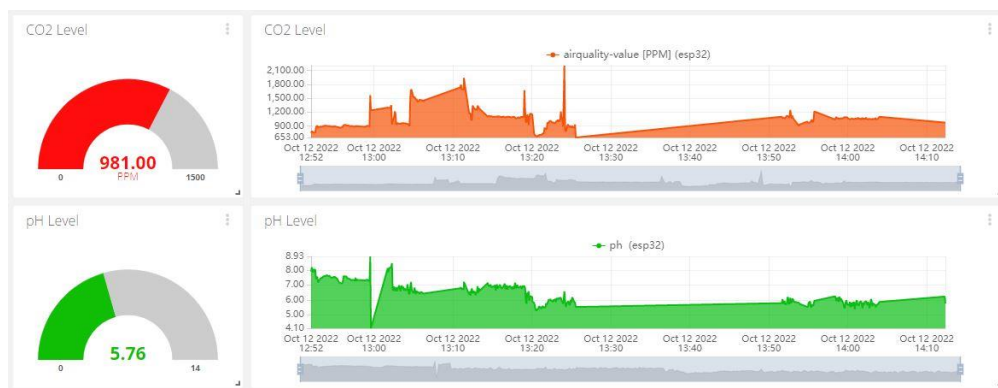
Figure 4.23: CO 2 and pH Level Monitor on Ubidots.
