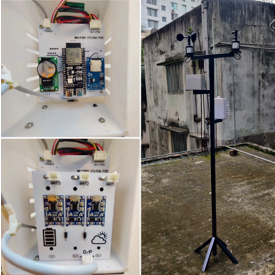
Fig. 6. PCBs placed inside the 3D printed protection box.
