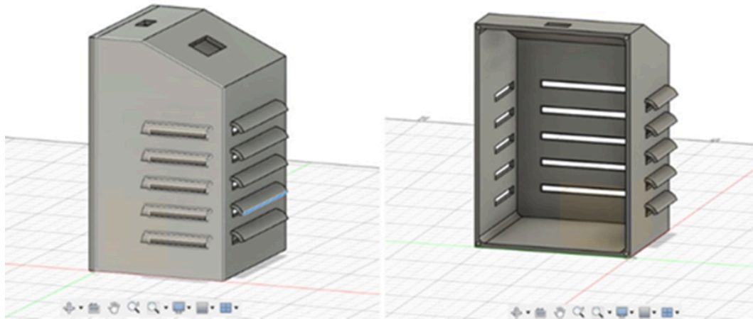
Fig. 4. Design of the 3D printed protection box.
