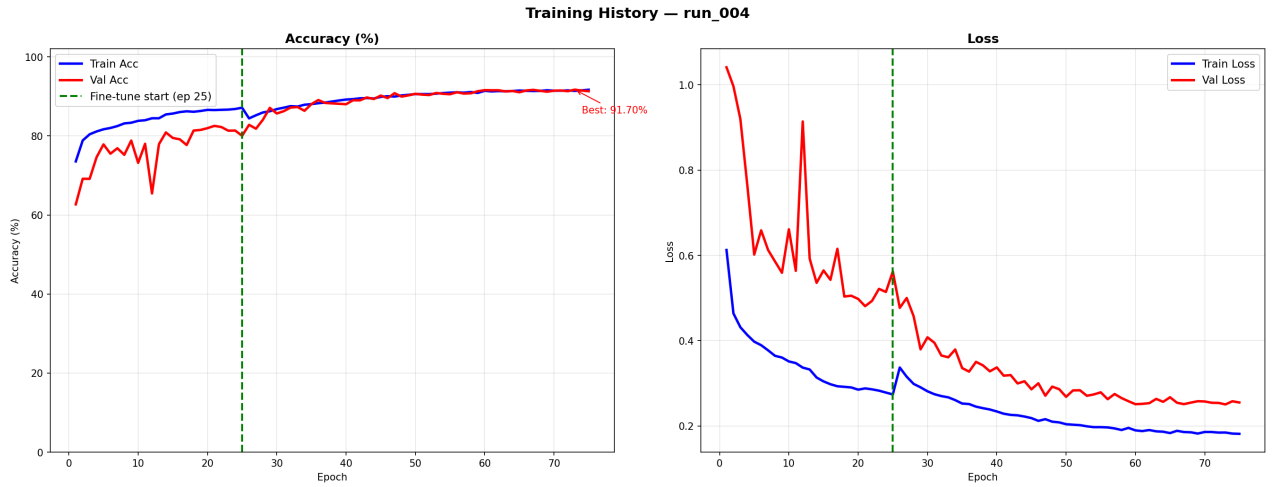
Figure 4.1: Training history — accuracy (left) and loss (right) across 75 epochs. The green dashed line marks the Phase 1/Phase 2 boundary at epoch 25. Best validation accuracy: 91.70 %.
