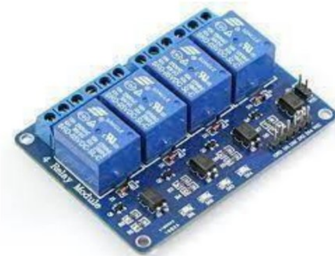
Fig- 3.12: Relay Module
