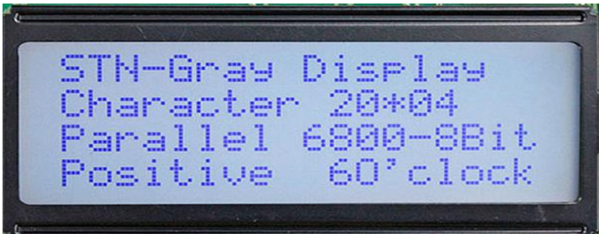
Figure 3.5: 20x4 LCD Display
