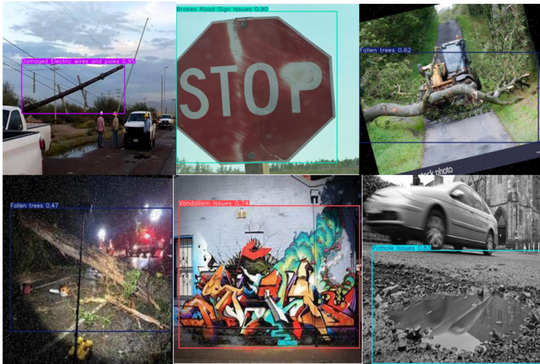
Figure 6.1: Model detection of urban infrastructure issues, including damaged electric wires, broken road signs, and potholes.
